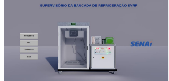
Fig. 5: SCADA system interface of the VRF bench showcasing enhanced monitoring and control capabilities.
